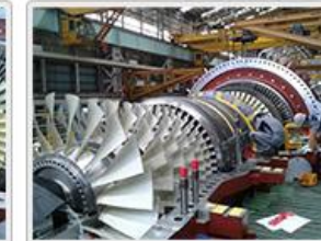
Blade Ring Assembly & Bolt Tightening
