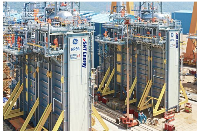
Heat Recovery Steam Generator
